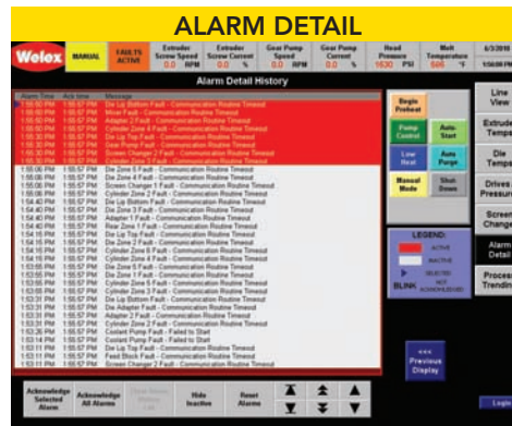
Detailed display of active alarm status, plus alarm history for all associated components in a single view. Clear descriptions provided for each event. Tiered alarms are color coded (warning, fault, or fatal), and can be selectively viewed by type.
