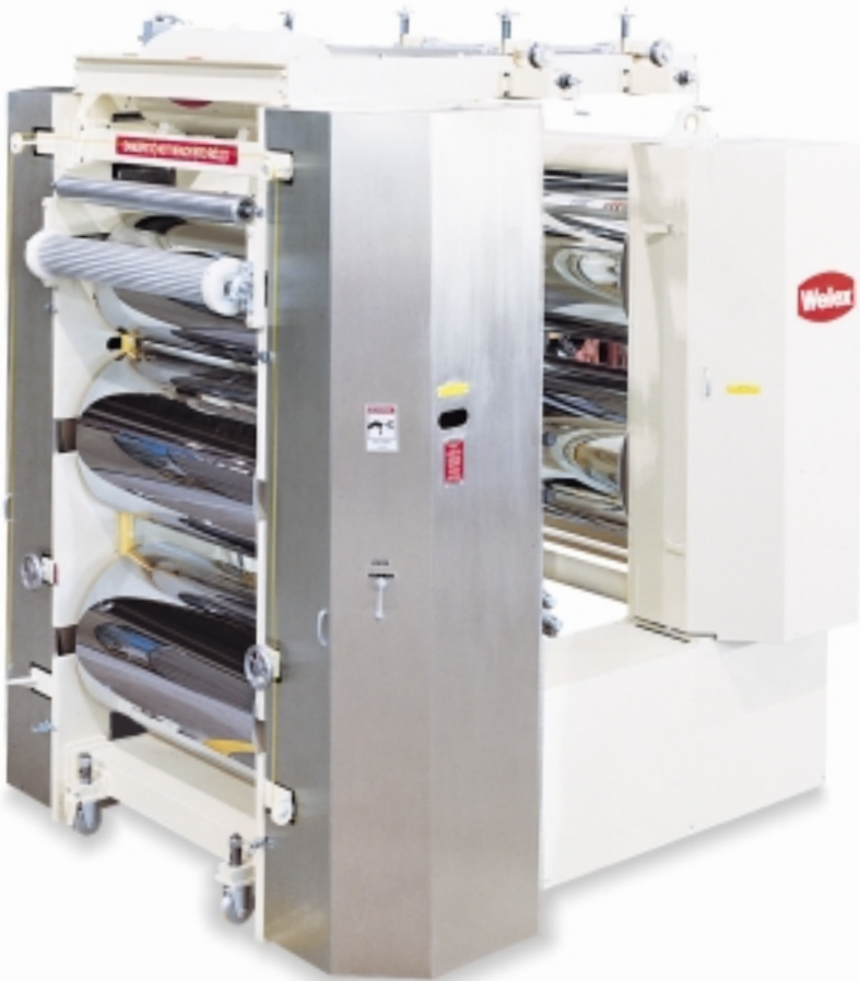
Additional cooling rolls Laminating pay-off
