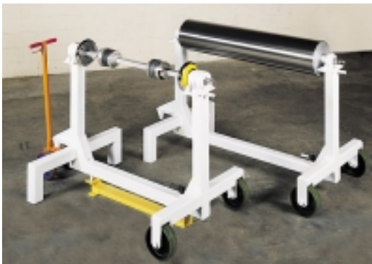
Removable and fixed shaft winding carts for jumbo roll winding system
